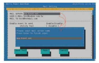
Use the directional key to select and press the Enter key to input data.
