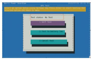
UPS Test includes: Self Test, Test to battery low and Cancel Test. Use the directional key to select the type of test. Then press the Enter key to execute or cancel test command. The screen display current test status and real time monitoring information. "Test in progress" indicates the machine is executing test command.
